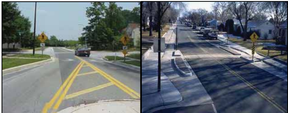
Figure 16 – Chokers at Pedestrian Crossings
