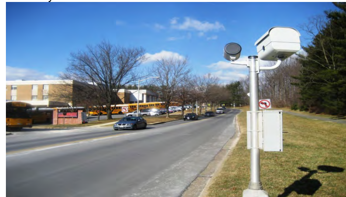
FIGURE 12 - 4. Speed Cameras. A speed camera unit is deployed on a local roadway in a school zone to help enforce posted speed limits and enhance pedestrian safety.
