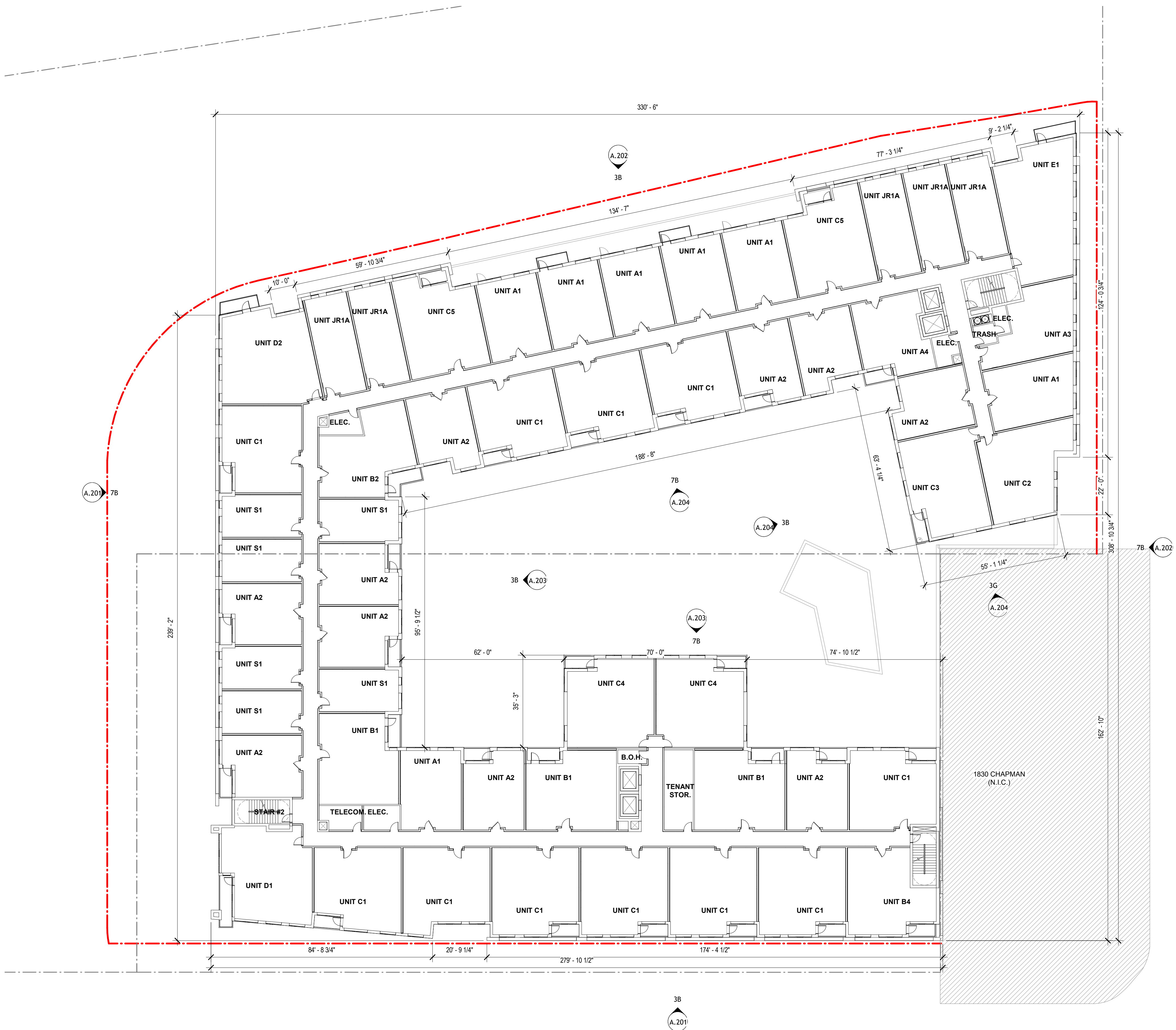
7B FLOOR PLAN - TYPICAL (LEVELS 5 - 8) A-201 A.105 1" = 20'-0"
