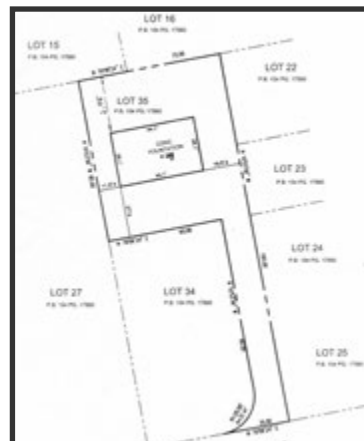
Figure 17. Example of pipestem lot
