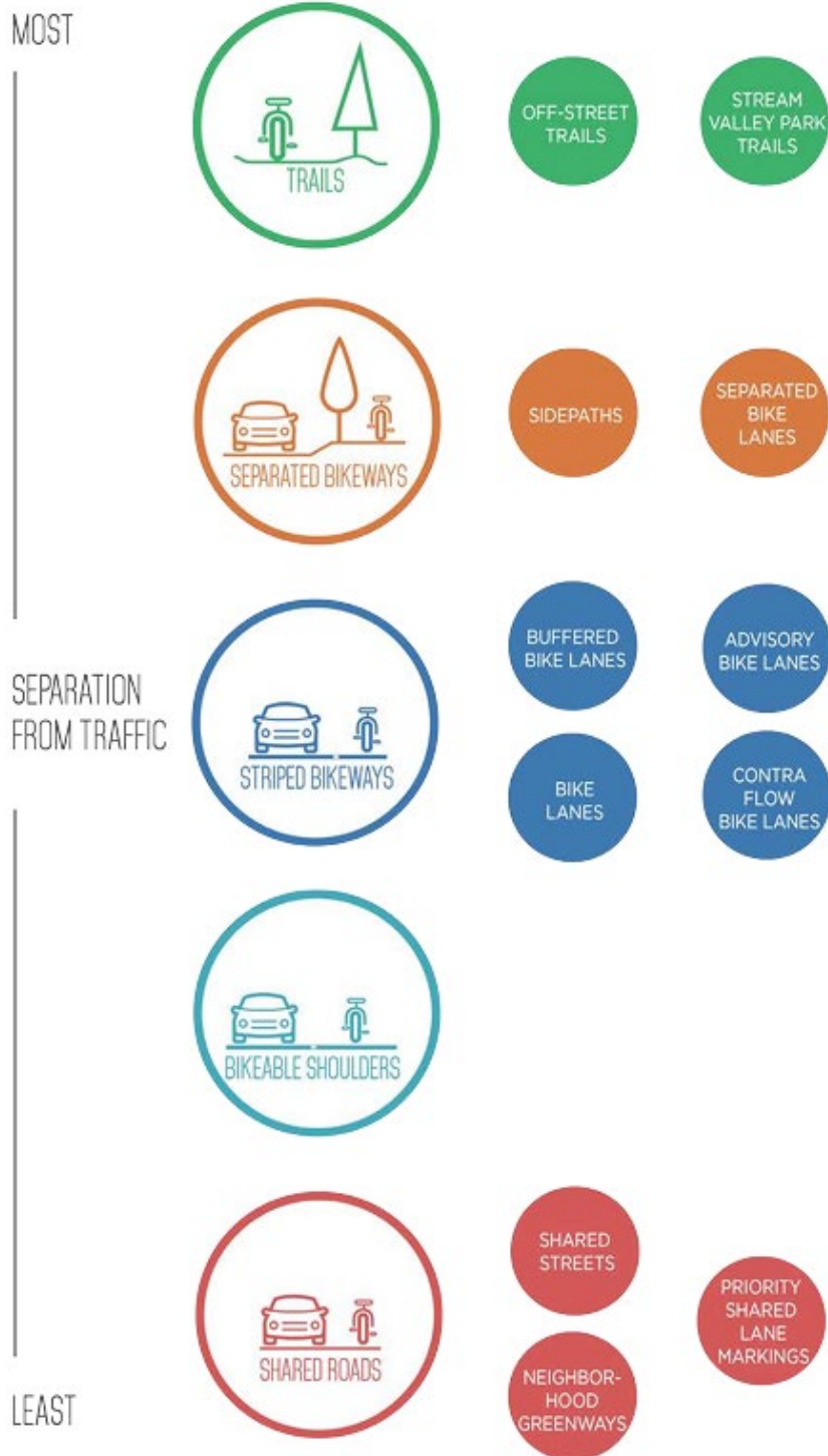
Figure 30 Bicycle Facility Classification
