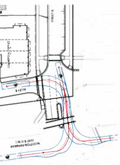
FIRE OUT FOR PERPENDICULAR ALLEY INTERSECTION (PRIVATE)
