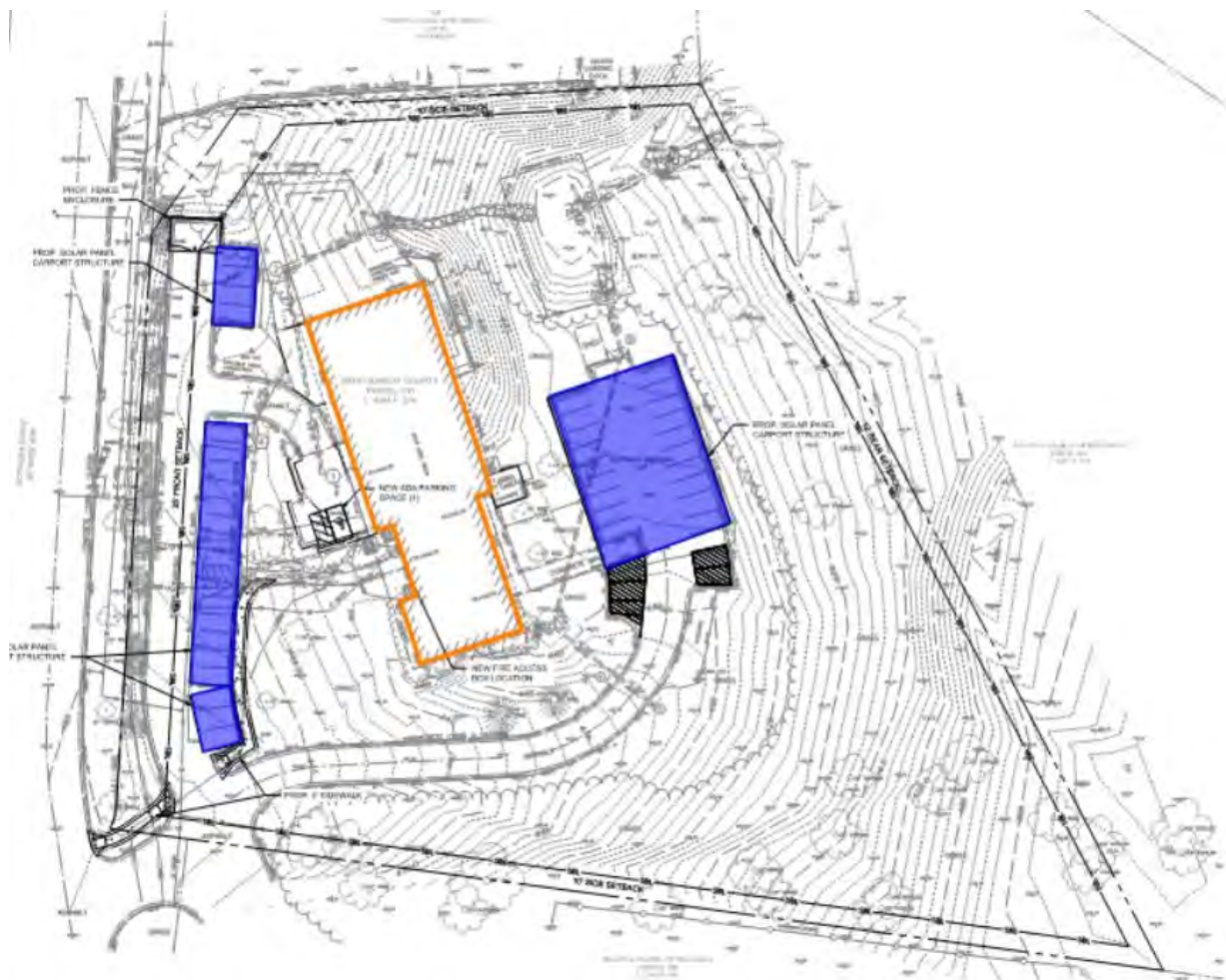
Proposed Site Plan with existing building outlined in orange and proposed solar carports shown in blue (site plan provided by applicant; markups by staff)
