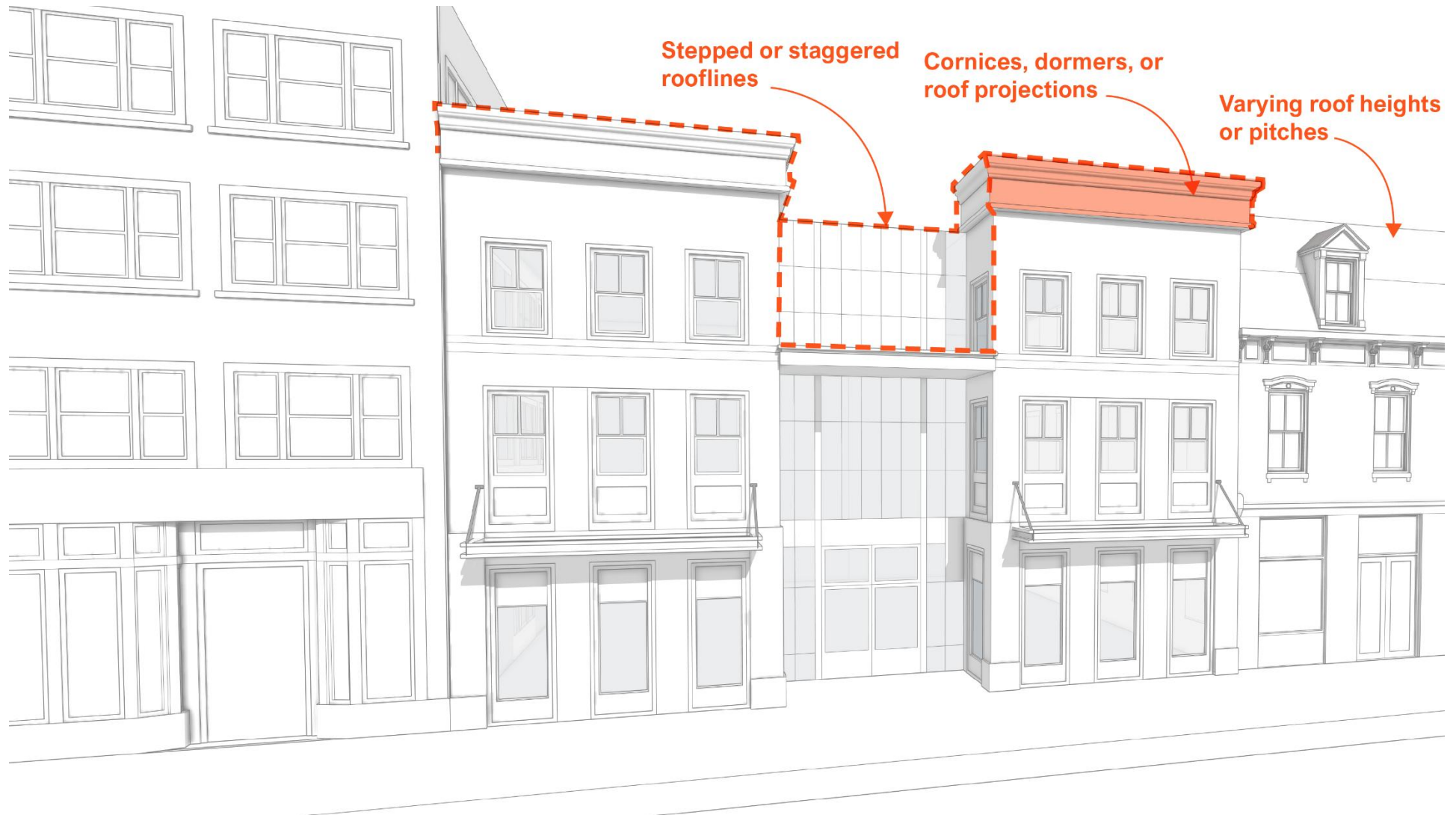
Figure 7.3.7-2: Mixed Use Design Standards – Roofs
